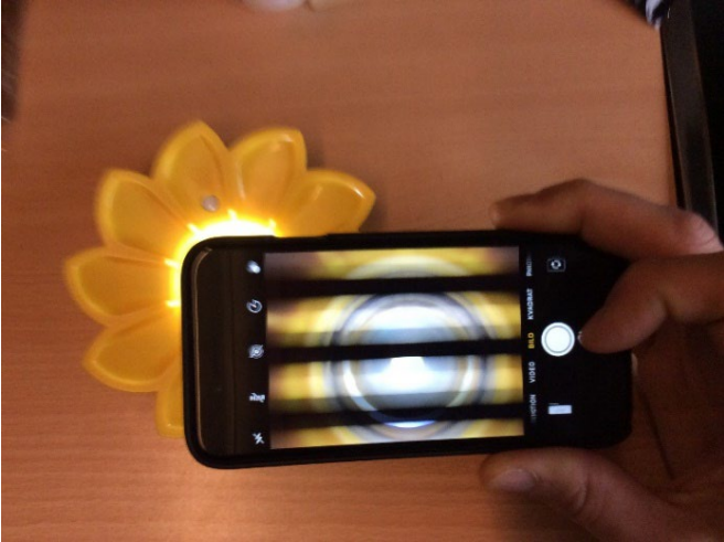
Mobile cameras use rolling shutter
